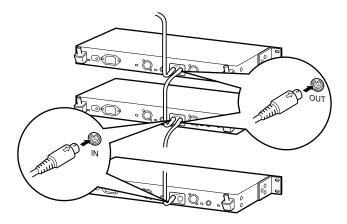
Then connect the "Remote Out" of the last UR6D or UR6DX receiver to the IF6P "1 In." If you are only using a single UR6D or UR6DX, connect its "Remote Out" to the IF6P "1 In."
